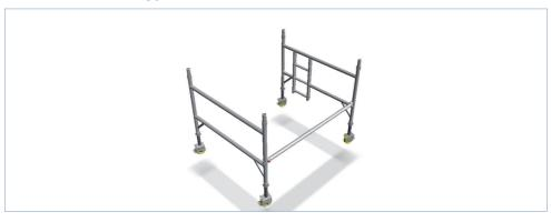
1.6 Clip the second brace in the same position. Make sure the base is level using a spirit level. If alterations are required do so by adjusting legs.
