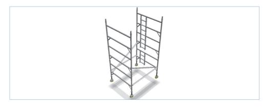
1.12 When fitting the stabilisers, position each one in opposing directions. Adjust all four castors to ensure the tower is square and level. Use a spirit level.
